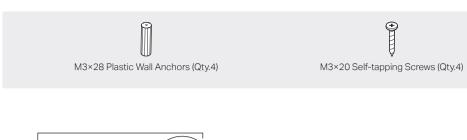
If your Ethernet cable feeds through the wall, you can position the mounting bracket below the cable hole. Mark four positions for the screw holes and then drill four 6 mm diameter holes at the marked
