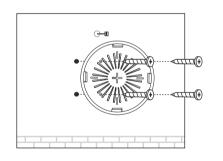
Secure the mounting bracket to the wall by driving the self-tapping screws into the anchors. Make sure that the shoulders of the mounting bracket are
