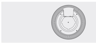
With the device powered on, press and hold the button for about 5 seconds until the LED flashes quickly . Then release the button. The device will restore to factory default settings.
